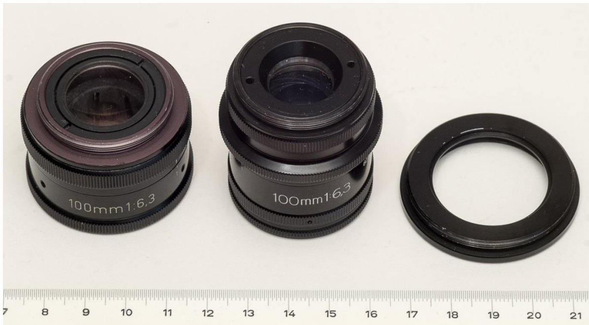
Fig. 18: Back view of the two 100mm Luminar versions. Left: the last version, a triplet construction, shows only two knurled rings, and has a 35mm thread. Center: the older version, an inverted Tessar construction, has 4 knurled rings and a 34mm thread; it often comes with an adapter ring to a 44mm thread (right).
