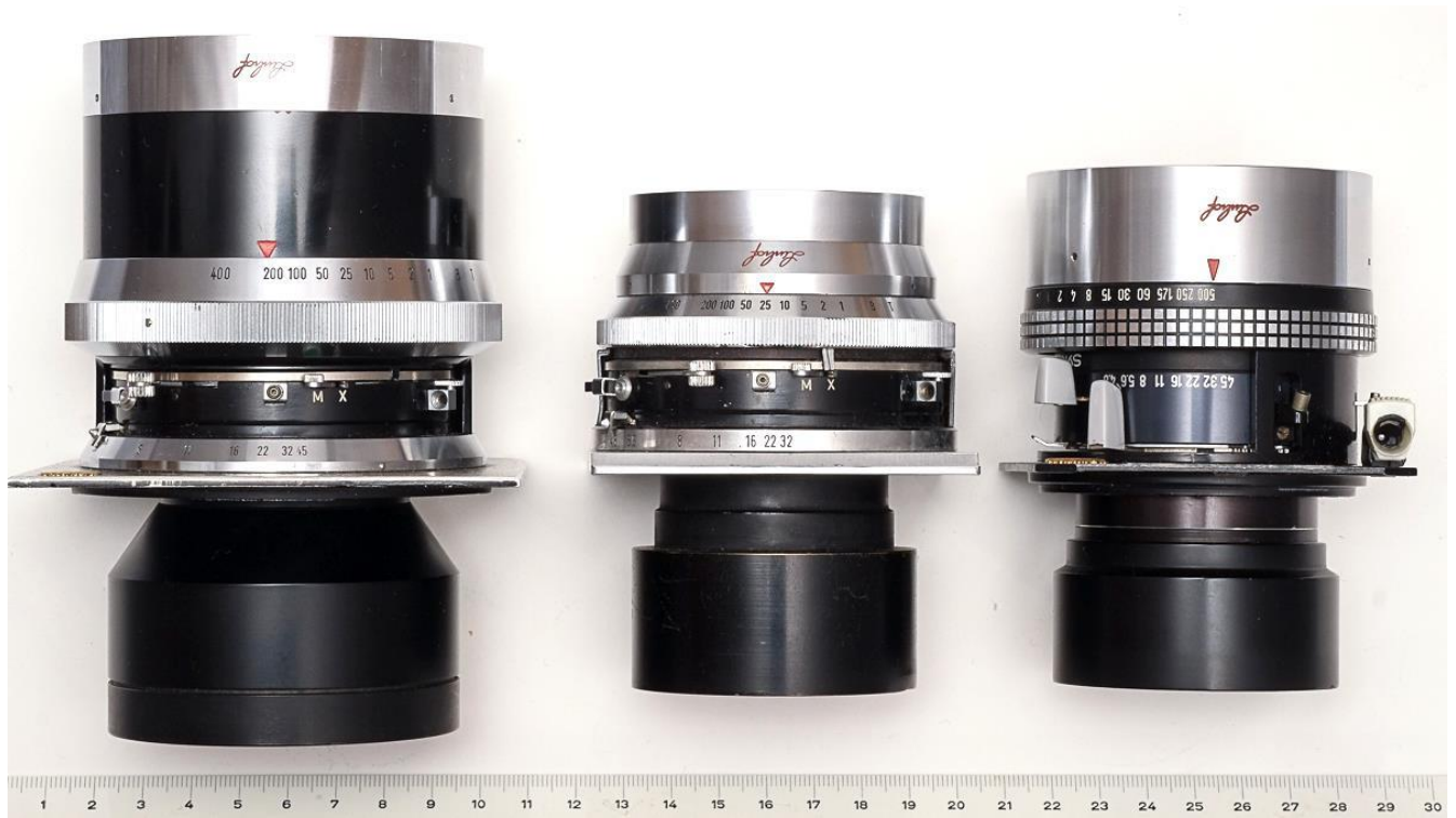
Fig. 9: Left, 250mm f/5.6 Sonnar with older style chrome plated shutter speed ring; center, older version of 180mm f/4.8 Sonnar in Synchro-Compur 1 shutter with chrome-plated cone-shaped front cell and shutter speed ring; right, newer version of 180mm f/4.8 Sonnar in Compur 0 with a design of small chrome-plated squares for the cylindrical shutter speed ring. Note the nonlinear aperture scales of the two older versions vs. the linear one of the new version on right. Scale is in cm.
