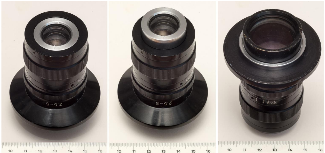
Fig. 20: The Zoom Luminar. Left: Front view, long focal length setting. Center: Front view, short focal length setting – the zoom is operated by the upper knurled ring. Right: Back view – note the much larger lens diameter compared to the front lens, and the chrome-plated annular dovetail connector for the Ultraphot II/III. See text for more details.
