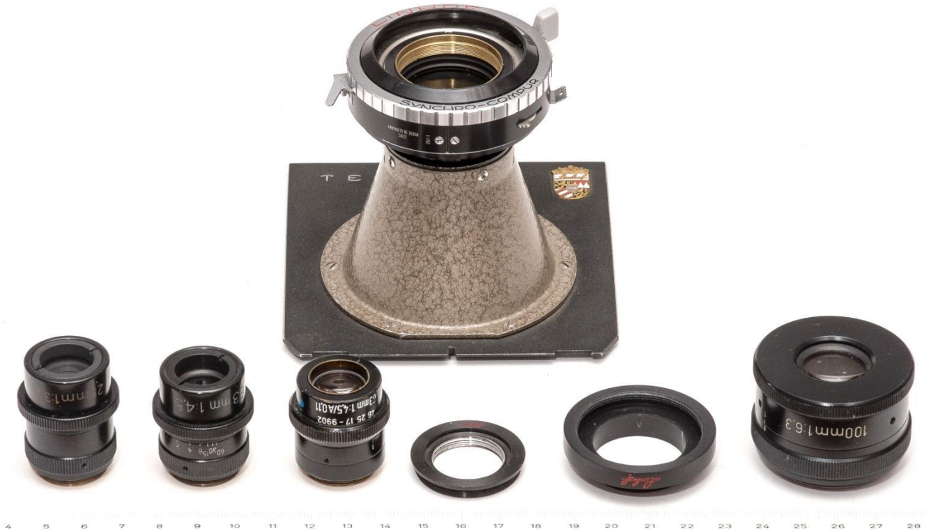
Fig. 15: Some Zeiss Luminars and the necessary accessories for LF photomacrography. Front row from left to right: Luminar 25mm f/3.5 (old version), Luminar 63mm f/4.5 (old version), Luminar 63mm f/4.5 (new version), Linhof adapter ring from RMS thread to size 0 shutter thread, Linhof adapter ring for M35x0.75 thread to size 0 shutter thread for the newer version of the 100mm Luminar, 100mm f/6.3 Luminar (last version). Back: Linhof adapter “cone” on Technika board with Compur 0 shutter for mounting the Luminars to a Technika or similar large format camera. Scale is in cm.
