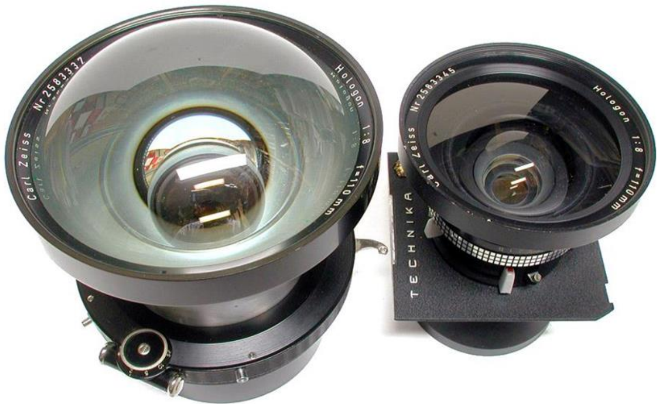
Fig. 22: Two prototype versions of the 110mm f/8 Hologon for 13x18cm/ 5x7". Left: First Version consisting of three thick lens elements with strongly curved outer surfaces, quite similar to the 15mm Hologon for 35mm film. The aperture was fixed to f/8, the shutter aperture could not be used. Right: Second version shown at 1966 Photokina, using 5 lens elements in 4 groups; the construction is closer to a Super-Angulon, although with thicker elements, and allows the use of the shutter's aperture. Image courtesy of Westlicht Photographica Auction [43].
