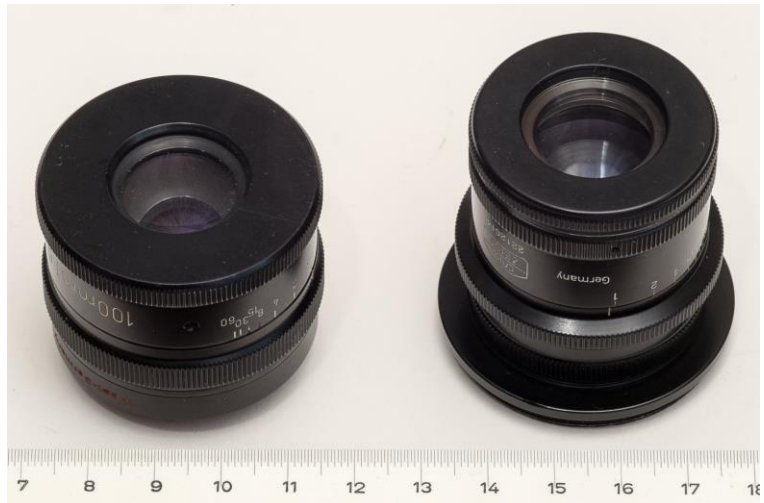
Fig. 19: The two versions of the 100mm Luminar, front view. Left: new version, right: old version
