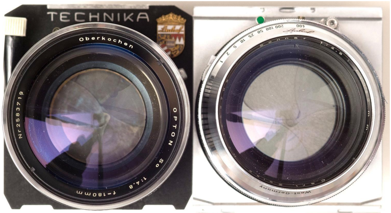
Fig. 8: Two versions of the 180mm f/4.8 Sonnar. On the left is the newer version with 67mm filter size and Compur 0 shutter; it is also an “Opton” version, note that the lens name is just “So”. On the right is the older version with 58mm filter size and Synchro-Compur 1 shutter, with the regular “Sonnar” and “Carl Zeiss” engravings. Note the steep angle of the engraved front ring of the right lens due to the small filter size.
